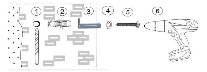
Check the Wall type before installation of dowel. Wall is drilled with equal diameter of dowel.(08mm) Universal Plastic Dowel provides the general purpose usage. Requires two stages assembly.
