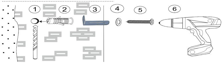
Check the Wall type before installation of dowel. Wall is drilled with equal diameter of dowel.(08mm) Universal Plastic Dowel provides the general purpose usage. Requires two stages assembly. Dowel can be different type according to the wall type. (e.g. Plaster Sheet Partition Wall, Gas Concrete, Hollow Brick Wall) If required, use appropriate dowels and screws.
