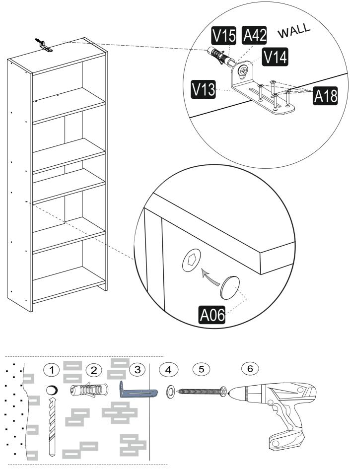
Check the Wall type before installation of dowel. Wall is drilled with equal diameter of dowel.(08mm) Universal Plastic Dowel provides the general purpose usage. Requires two stages assembly. Dowel can be different type according to the wall type. (e.g. Plaster Sheet Partition Wall, Gas Concrete, Hollow Brick Wall) If required, use appropriate dowels and screws.
